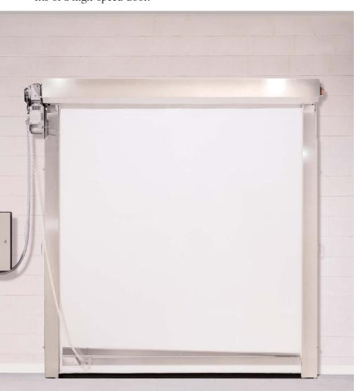
Sanitary Design - Classified by Underwriter's Laboratories (UL® 2128) to meet USDA hygienic standards for meat, poultry, dairy and seafood applications. The entire door is designed to be spray washed, yet its sanitary design prevents liquid contaminants from dripping into the traffic pathway and virtually eliminates potential sites for bacteria manifestation.
