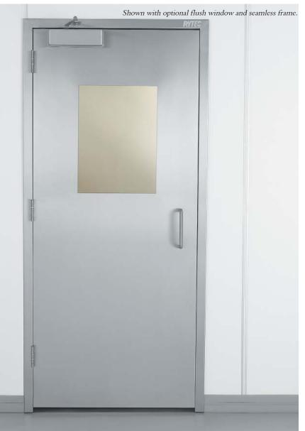
**Panel Construction** - Seamless, 16 gauge stainless steel skin with optional 18, 14 and 12 gauges. Panel uses 14 gauge reinforcing channels with a polystyrene foam core. Other core options include polypropylene honeycomb.
