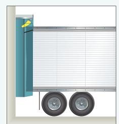
When vehicle is in position at the dock, the helical torsion springs of the product head member provides consistent tension force over the width of the unit while ensuring the foam head member conforms to the top of the trailer creating a watertight wiper seal.
